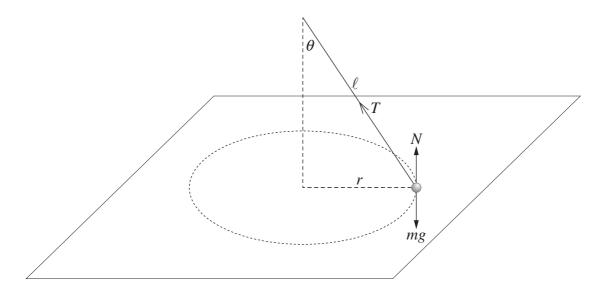
The particle remains in contact with the horizontal surface.
